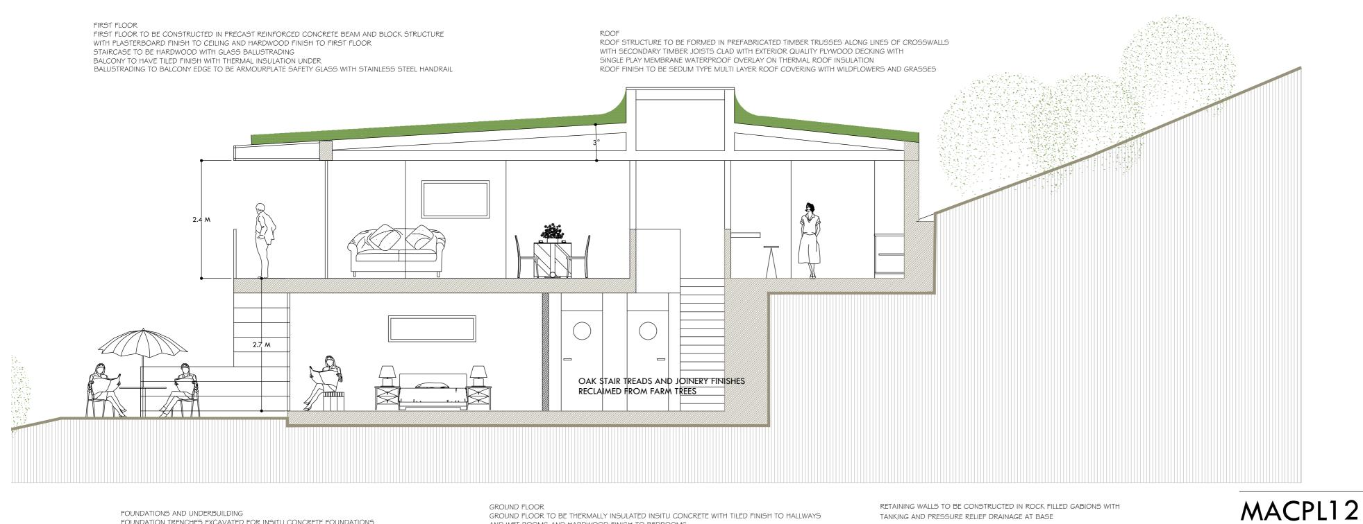
FOUNDATIONS AND UNDERBUILDING FOUNDATION TRENCHES EXCAVATED FOR INSITU CONCRETE FOUNDATIONS UNDERBUILDING TO BE DENSE CONCRETE BLOCKWORK RETAINING WALLS TO BE FORMED IN GALVANISED WIRE GABIONS FILLED WITH CRUSHED ROCK FACED WITH DAMP PROOF MEMBRANE AND DENSE CONCRETE BLOCK FACINGS
